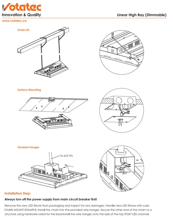
Make sure the wiring hangers are fully engaged into the side holes on the top channel.
